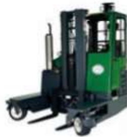
C Serie 4-Wege Allrad Stapler für Indoor-und Outdoor Langguttransporte
